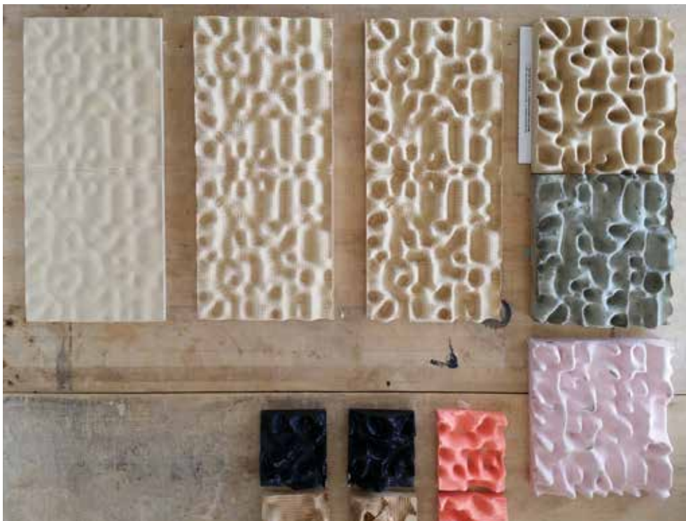
Figure 8. Final series of low to high relief panels cut for aquarium experiment - MDF, concrete and silicone panels shown at right. Additional featureless concrete panels (not shown) were cast as baseline for comparison in the study to simulate typical seawall conditions.
