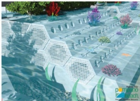
Rendering of SEAHIVE installation at Wahoo Bay including the modular concrete structures and mangroves to be planted on them.
